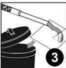
Dispense the initial amount of material from the mixing nozzle onto a disposable surface until the product is a uniform gray color with no streaks, as adhesive must be properly mixed in order to perform as published. Dispose of the initial amount of adhesive according to federal, state and local regulations prior to use. **CAUTION:** When changing cartridges, never re-use nozzles. A new nozzle should be used with each new cartridge and steps 1 - 3 should be repeated accordingly.
