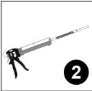
Screw on the proper Adhesives Technology mixing nozzle to the cartridge (see Table 1) after properly balancing the cartridge. Do not modify mixing nozzle. Confirm that internal mixing element is in place prior to dispensing adhesive. Take note of the air and base material temperatures and review the working time (see Table 3) prior to starting the injection process.
