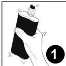
**Shake the cartridge vigorously for 60 seconds**, then stand cartridge upright for at least 1 minute allowing any bubbles to rise to the top.
