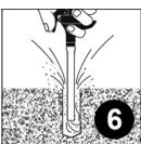
Blow out and remove all dust, dirt, debris, oil and any other contaminant from the control joint or crack. Use backer rod or kiln dried sand prior to application of adhesive. Allow sufficient depth for joint filler based upon minimum recommended depth of filler. Place mixing nozzle directly over the joint or repair area. Dispense material using full smooth trigger pulls (no short, choppy strokes) and allow material to gravity feed into the crack/joint.
